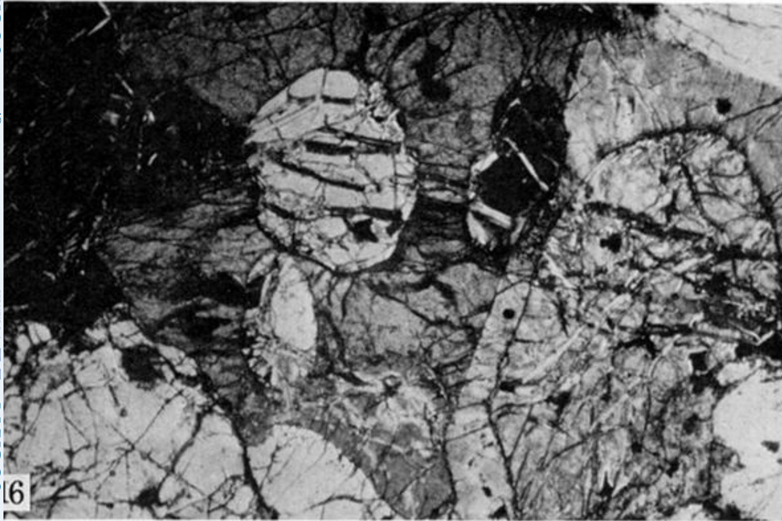
FIGURE 16. Thin section of cumulate-textured olivine pyroxenite. Subhedral olivine, anhedral, twinned, poikilitic augite. Crossed Nicols, max. dimension 3.2 mm.
