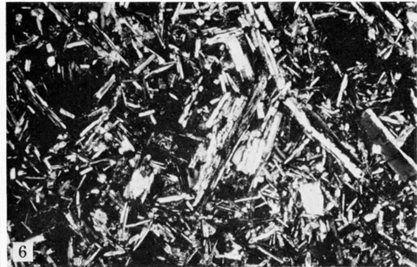
FIGURE 4. Photomicrograph of Upper Pillow Lava rock. Phenocrysts are calcite replacements of olivine in microcrystalline to glassy altered groundmass. Plain light, max. dimension 1.6 mm.
